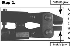
Open tool jaws and insert inside jaw into the fitting so that the outside (cutting) jaw is positioned over the crimped ring. Close the tool jaws.
