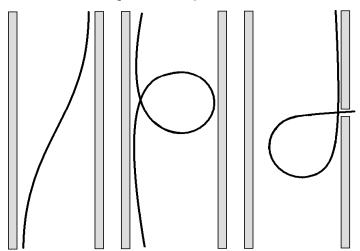
Since Everhot PEX will expand and contract  $\sim$ 1" for every 100ft of tubing at a  $10^{\circ}$ F temperature change, a proper slack must be provided to offset such thermal changes. For longer pipe runs the later can be done by making a loop or an offset as shown on the picture (left).
